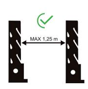
Place brackets the way that maximum horizontal spacing between them is 1,25 m
